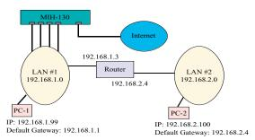
To achieve the static route in the example above, the following information would be inputted into the Static Routing page of the XRouter Pro:
